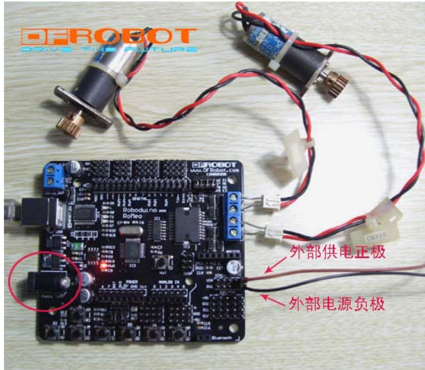
Figure 4 Romeo Motor Connection Diagram
