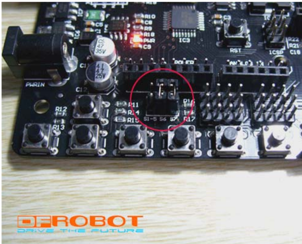
Figure 3 Button Enable Jumpers
